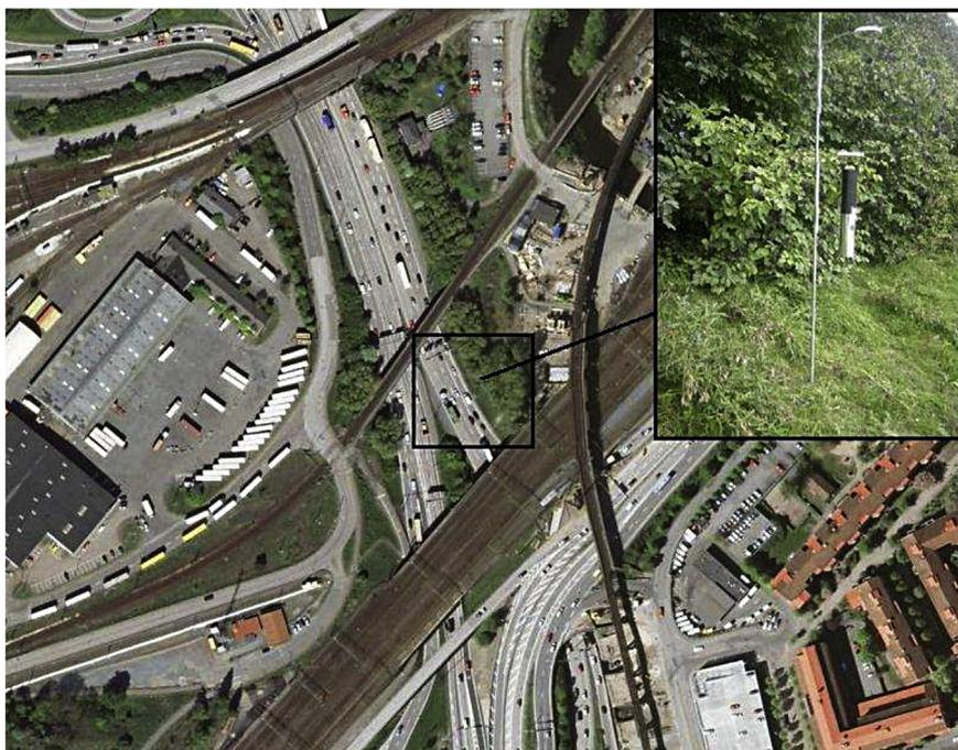
Fig. 1. Aerial view of the measurement site in the City of Gothenburg, south-west Sweden as well as a photo of the measurement site showing the measurement point outside the canopy and the forest edge inside which the measurement point inside the canopy was situated. The two measurement points were 4 m apart.
